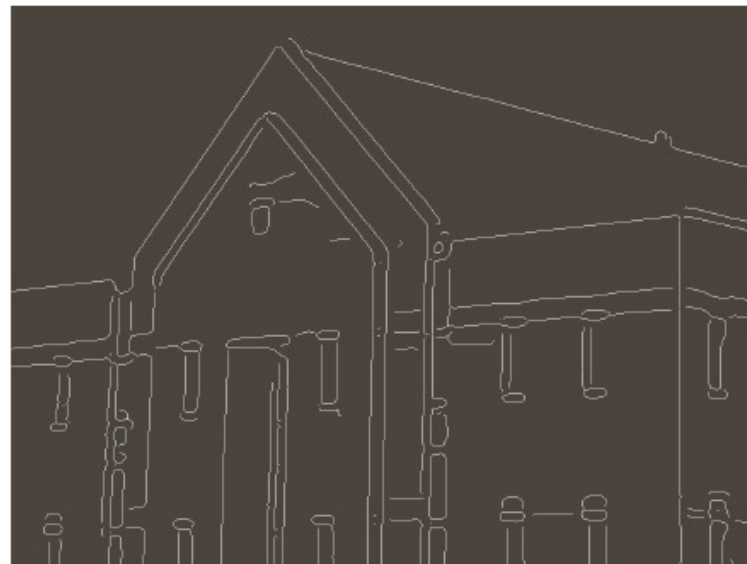
FIGURE 10.25 (a) Original image of size 834 \times 1114 pixels, with intensity values scaled to the range [0, 1] . (b) Thresholded gradient of smoothed image. (c) Image obtained using the Marr-Hildreth algorithm. (d) Image obtained using the Canny algorithm. Note the significant improvement of the Canny image compared to the other two.
