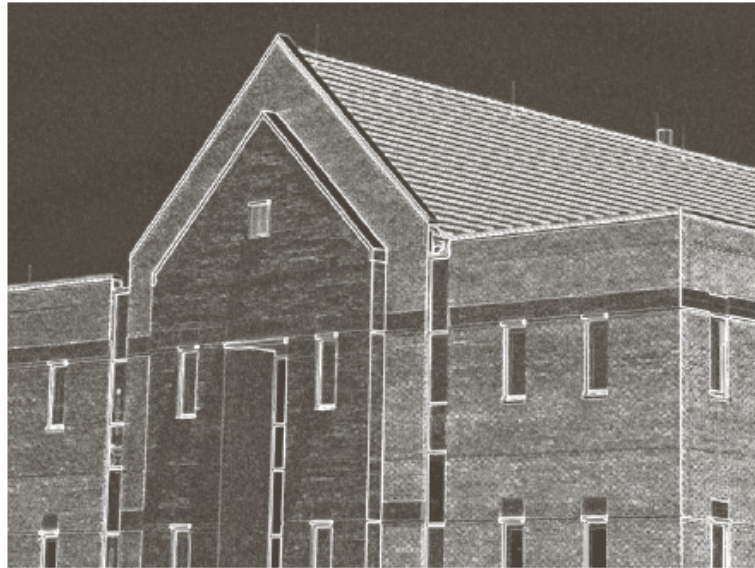
FIGURE 10.16 (a) Original image of size 834 \times 1114 pixels, with intensity values scaled to the range [0, 1] . (b) |g_x| , the component of the gradient in the x -direction, obtained using the Sobel mask in Fig. 10.14(f) to filter the image. (c) |g_y| , obtained using the mask in Fig. 10.14(g). (d) The gradient image, |g_x| + |g_y| .
